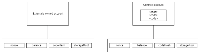
Fig. 3. Architecture of externally owned account (EOA) and contract account
