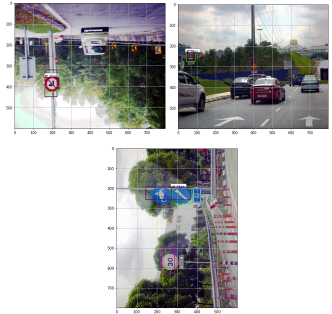
Fig. 4. The output of data generator, green box is ground truth box and purple box is anchor box
