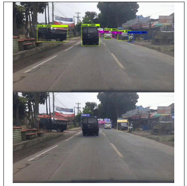
Fig. 5. Comparison of object detection (top) and object tracking (bottom) on the YOLOv4 416x416 model
