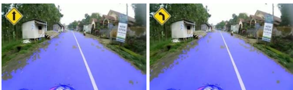
Figure 9. Effect of noise on determining the direction of the road.
