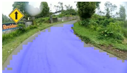
Figure 10. Detection of end of road failed (should be turn left instead of straight).
