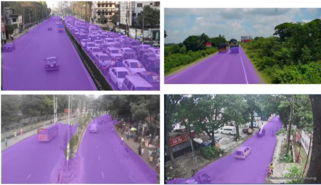
Fig. 3. Examples of road segmentation result
