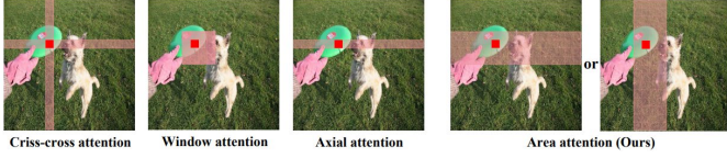
Fig. 5. Comparison of area attention with other attention mechanisms. Adapted from [6]
