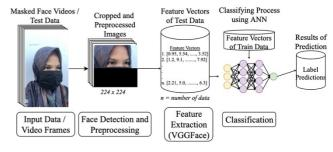
Fig. 3. System flow of testing scheme.
