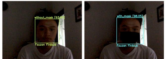
Fig. 8. Experimental results on a webcam with low-light condition.
