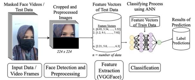
Fig. 3. System flow of testing scheme.
