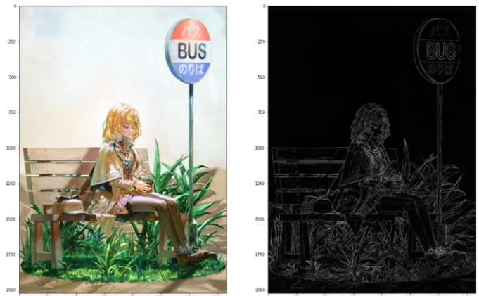
Figure 2: Left: Original image, Right: Applied Sobel filter to grayscale version of the original
