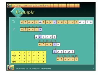
The first step is we have to find the boundaries function of each index of the pattern. The pattern that we would like to search in this case is "abacab". From the left-down side of the picture above, we can see the boundaries function of the pattern. Here is the step by step to determine the boundaries function(b(k)):
