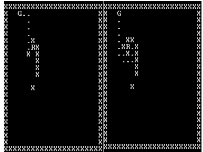
Figure 7 . The Robot encounters an obstacle in its original path and replan the path starting from the current position
