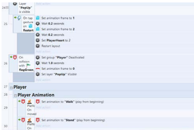
Fig. 4. Event System (with subevents, conditions, actions, triggers, and groups)
