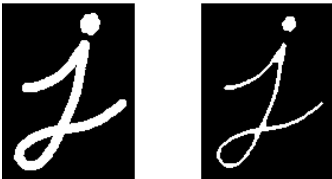
Figure 3 Erode a frame
