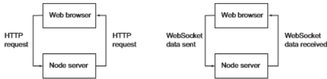
Figure 2. Serving HTTP and WebSocket using a single TCP/IP port [2]
