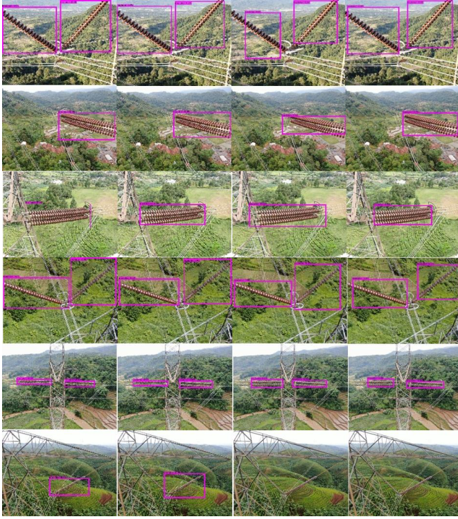
Fig. 5. Detection results in PLN dataset, from left: YOLOv2, our baseline network, YOLOv3-tiny, SF-YOLO. Enlarge the digital document for clarity.
