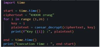
Fig. 8. Python Implementation to decrypt Caesar Cipher by testing all available key combination.
