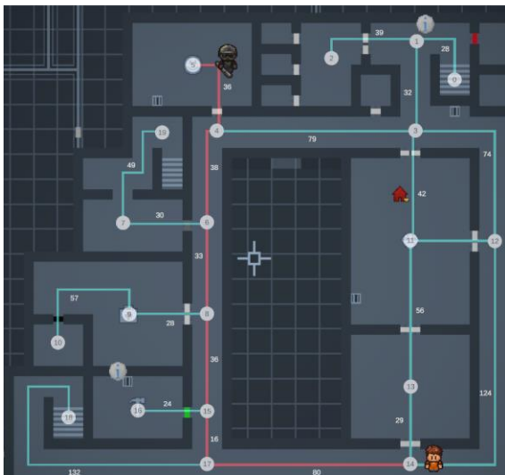
Fig. 16. The shortest path generated by Dijkstra's algorithm from room 5 to room 14
