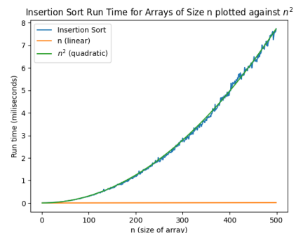
Figure 10, Insertion sort run times for array of size n Source: writer's analysis
