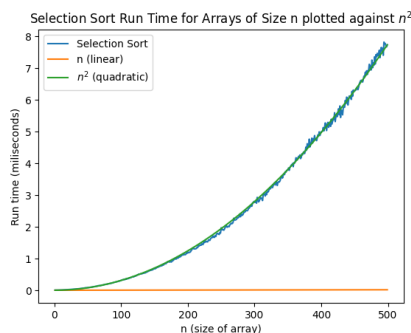
Figure 9, Selection sort run times for array of size n Source: writer's analysis
