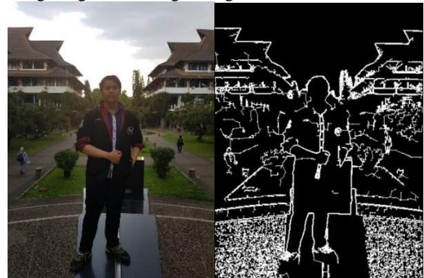
Figure 5. Example of before (left) and after (right) edge detection with epsilon 20 and thresDest 30. Photo taken by author in Plaza Widya Nusantara ITB.
