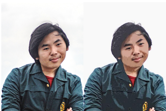
Figure 6. Example of before and after cutout filter based on Image Segmentation with threshold 60 and radius 3. The result is both better and worse than the Adobe Photoshop's cutout in each of its aspect.
