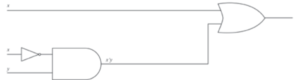
Figure 18. Circuit representation of variable A
