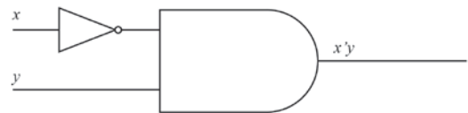
Figure 19. Circuit representation of variable B
