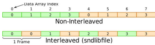
Fig. 5. Non-interleaved and interleaved audio with two channels Source: The Lab Book Pages
