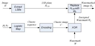
Fig. 2. Block diagram of watermark embedding
