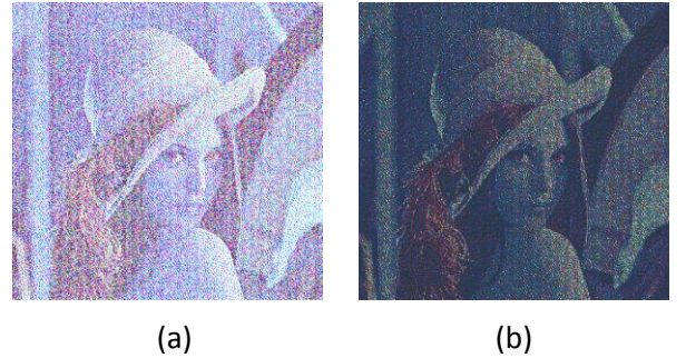
Figure 5. The result of stacking shares generated with (a) RGB and (b) CMY color model
