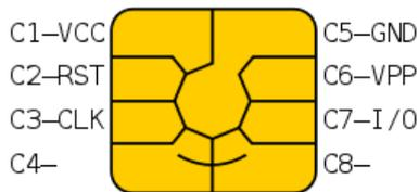
Gambar 1. Ilustrasi *chip smart card*
