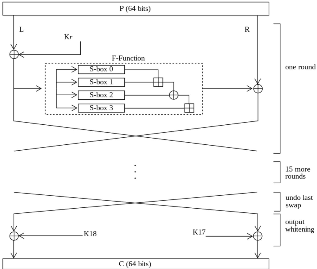
P=Plaintext; C=Ciphertext;  $K_x$  = P-array-entry  $x$
