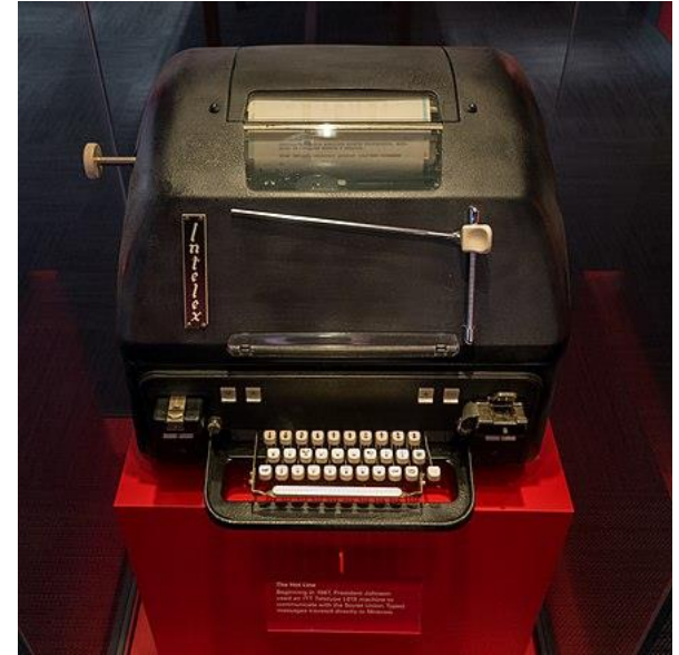
ITT Intelex Teletype L015 used for original Moscow–Washington hotline (Lyndon Baines Johnson Library and Museum)
