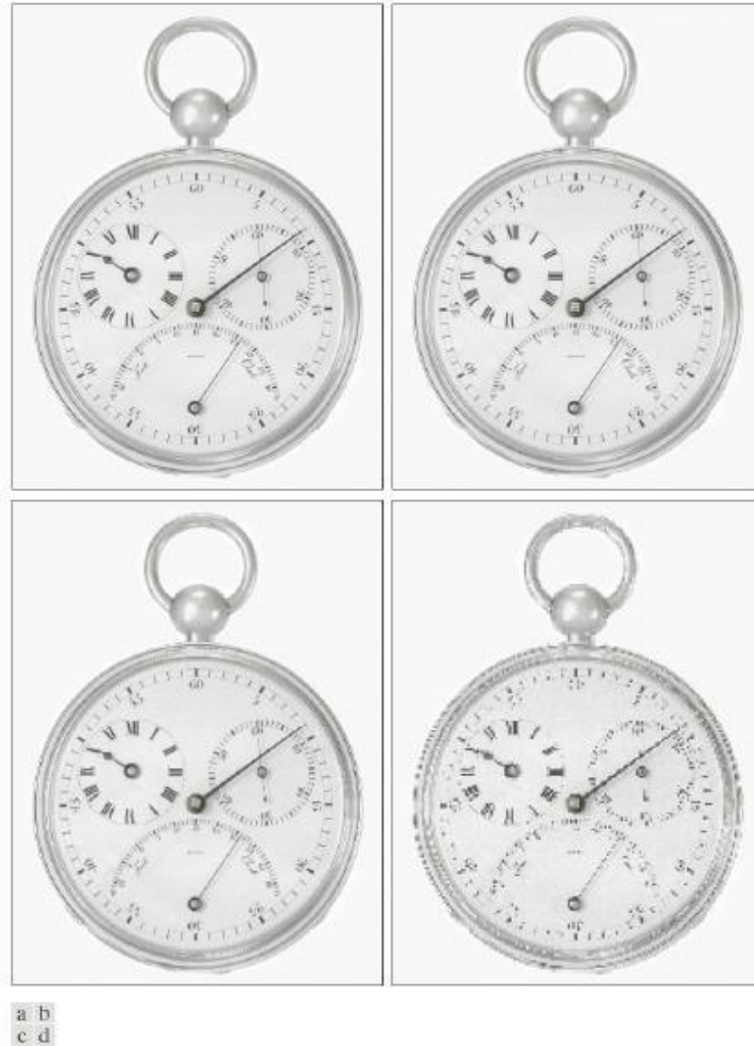
FIGURE 2.20 Typical effects of reducing spatial resolution. Images shown at: (a) 1250 dpi, (b) 300 dpi, (c) 150 dpi, and (d) 72 dpi. The thin black borders were added for clarity. They are not part of the data.
