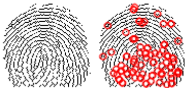
Image II.8. Keypoints generated by SIFT algorithm for fingerprint matching
