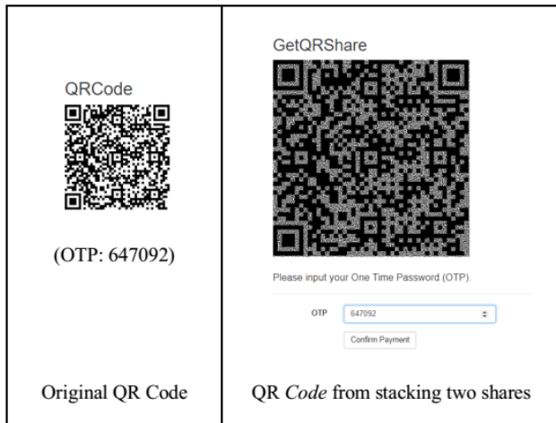
Fig. 14. An example of the original QR Code and the QR Code resulted from stacking two shares
