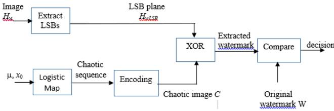
Fig.3. Block diagram of watermark extraction.
