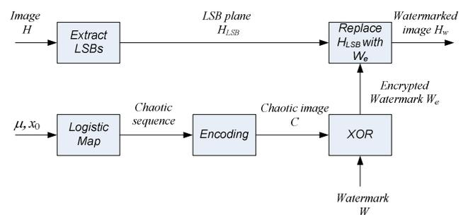
Fig. 2. Block diagram of watermark embedding
