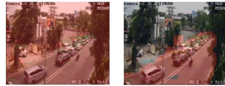
Figure 9. Detection Result without and with Region of Interest Extraction. (Left: without RoI extraction. The false positives: the cars parked on the left side of main road and on far road on top is counted. Right: with RoI extraction. The false positives are not counted.)
