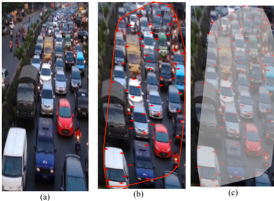
Figure 6. System testing: (a) Traffic congestion; (b) corner reading; (vertices), marked by the ‘+’ signs on objects’ corners
