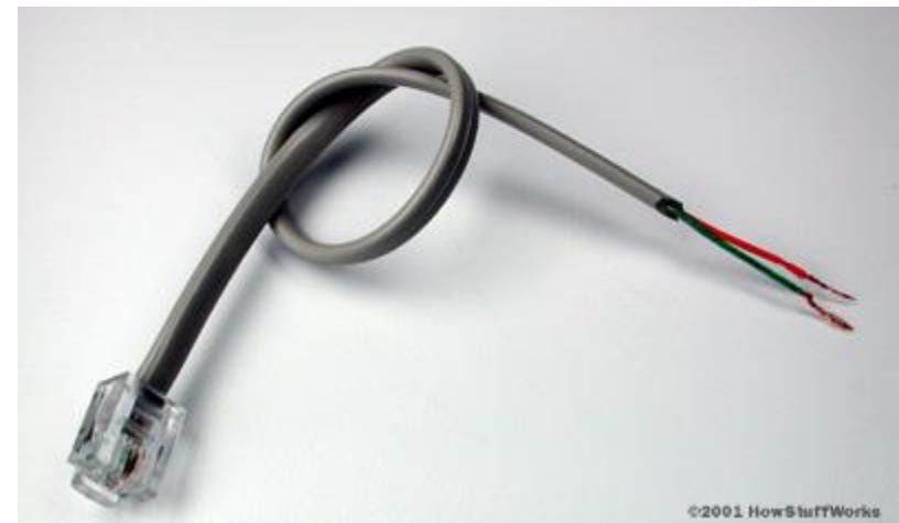
**Inside a standard phone cord, you'll find a red wire and a green wire. These wires form a circuit like the one you might find in a flashlight. Just as in a flashlight, there is a negatively-charged end and a positively-charged end to the circuit. In a telephone cord, the green wire connects to the positive end and the red cord connects to the negative end.**
